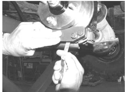
Fig. R7 - Check pad clearance
