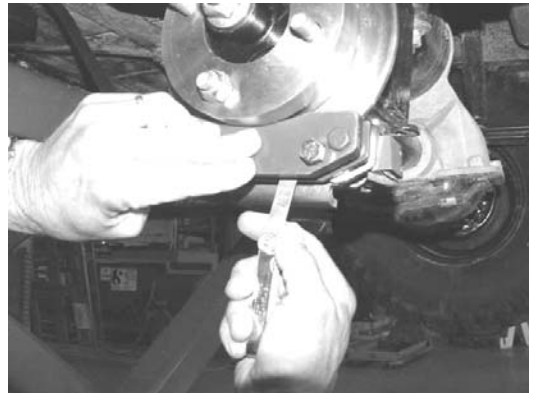
Fig. 16 Check pad clearance of both wheels at the same time.
