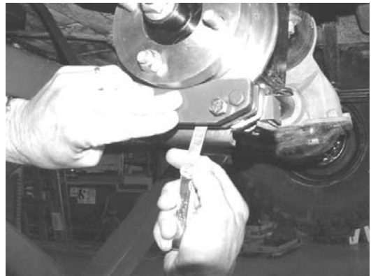
Fig. M3 - Check pad clearance of both wheels at the same time.
