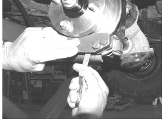
Fig. R11 - Check pad clearance of both wheels at the same time.
