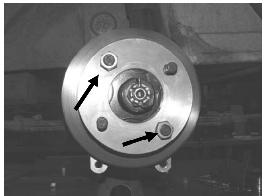
Fig. 7 - (2) lug nuts to temporarily hold rotor in place.
