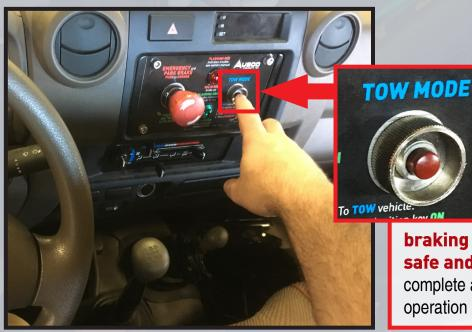
Tow Mode allows a disabled vehicle to be moved safely without hand pumps or jumpers. The operator can release the brake from the safety of the driver's seat with all
